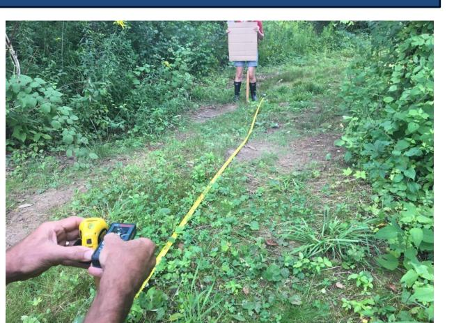
The team recorded ground height using a laser measuring tool, as well as the distance between two waypoints to calculate slope of areas in need of immense work.
