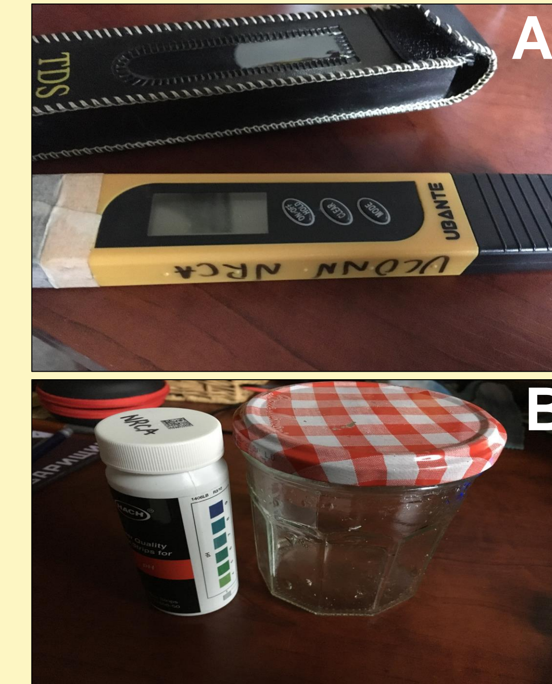
Figure 2. A: Ubante TDS Meter for water quality testing; B: pH strips and jar used to collect water samples
