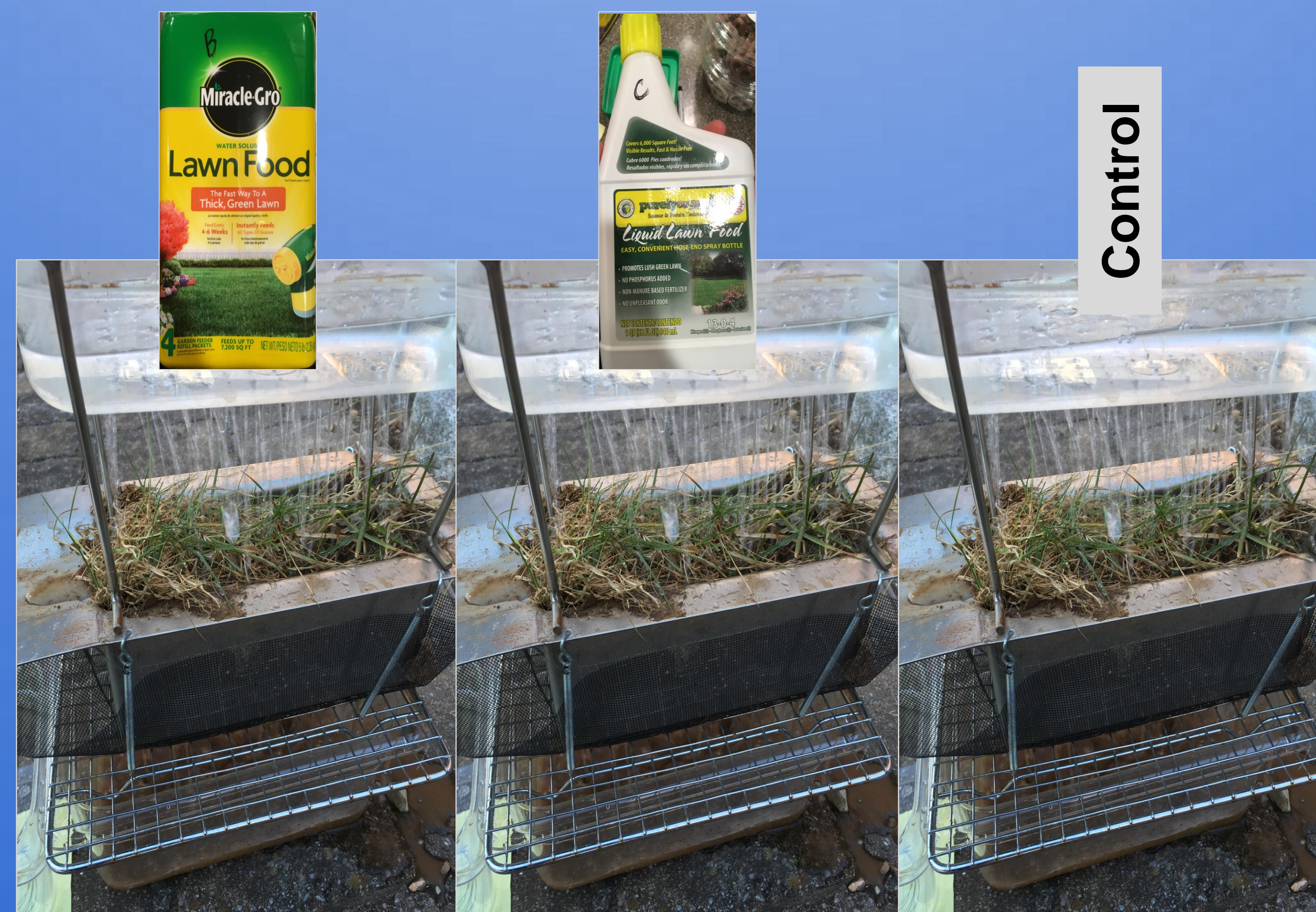
Fig 2. Three rain simulators comprised three parts each: an upper basin with holes, a planter base with local grass and soil, and a lower basin with LIS water. In two of the simulators fertilizer (Miracle-Gro Water Soluble Lawn Food or Purely Organic Liquid Lawn Food) and tap water were placed in the upper basin, and in the third simulator, no fertilizer was included in the tap water in the upper basin (control).
