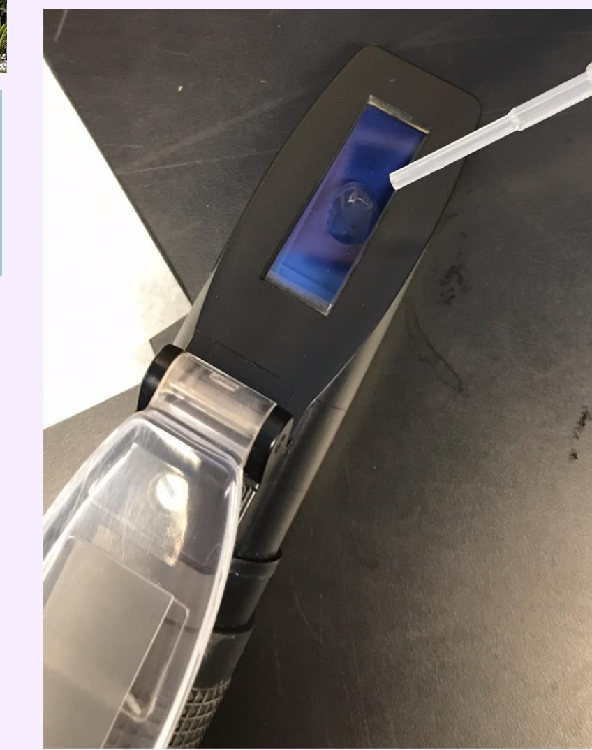
Fig. 5 : Soil solution being placed into the refractometer.
