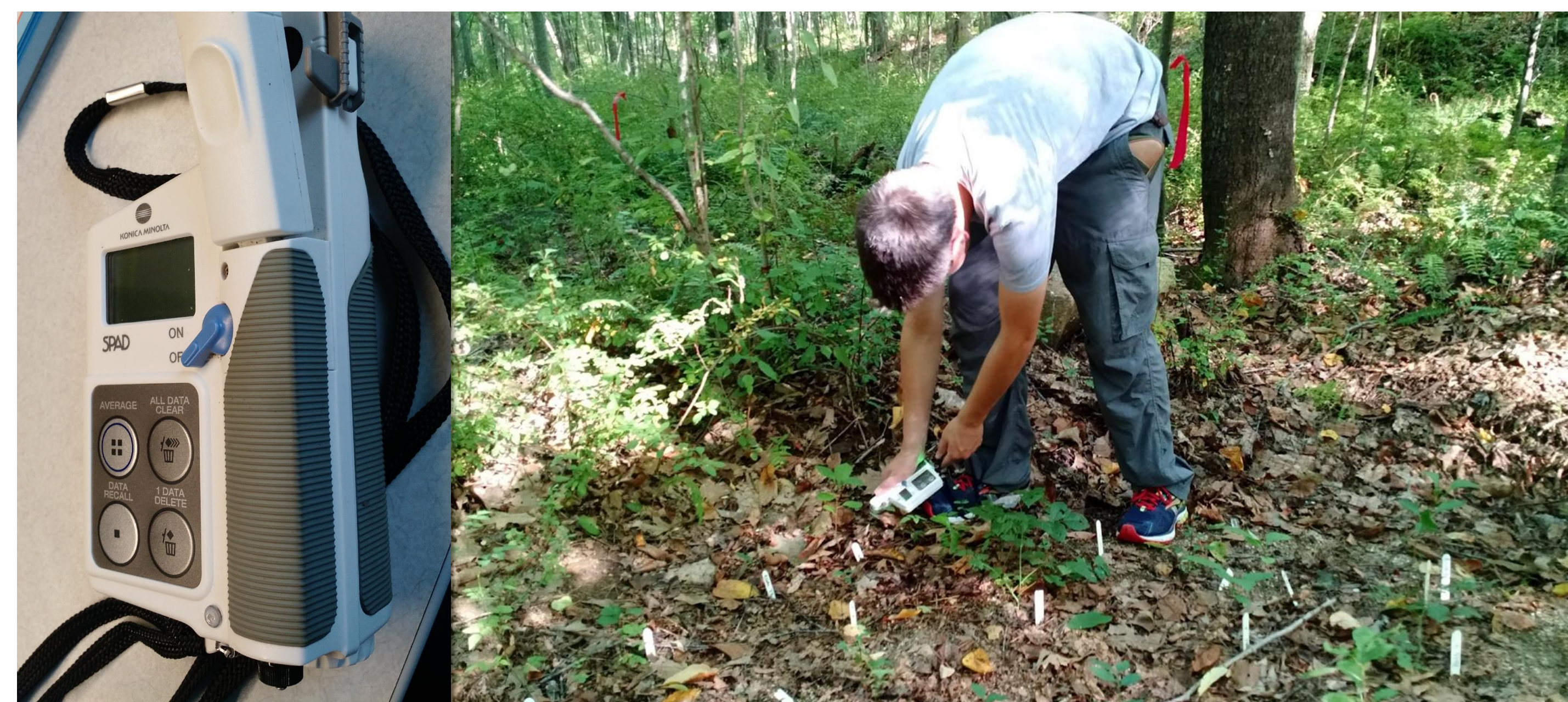
Fig 2. (Left) The chlorophyll meter. (Right) Use of the chlorophyll meter within a test site.
